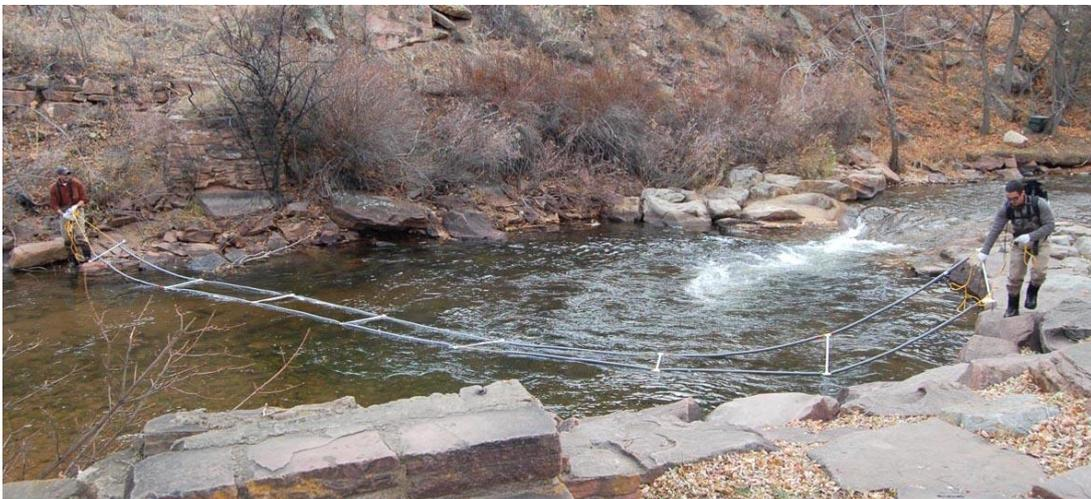
Figure 6 Floating antenna, hand-carried
