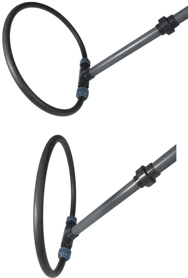
The loop orientation can be changed depending on the expected orientation of the PIT tag. If multiple tags are in random orientations, the area should be scanned at different orientations to make sure they are all detected.
