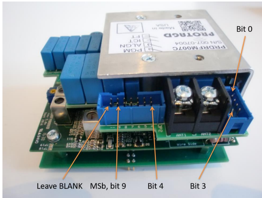
Figure 5.3 Jumper for Antenna Tuning
